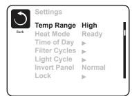
High Range can be set between 80°F and 104°F. Low Range can be set between 50°F and 99°F. More specific Temp Ranges may be determined by the Manufacturer. Freeze Protection is active in either range.
