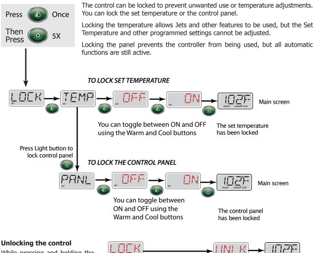
While pressing and holding the WARM Button, press the LIGHT button twice.
