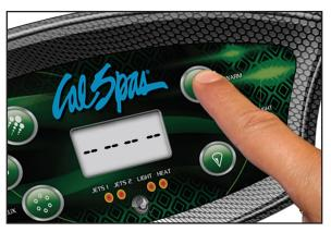
Your spa will perform a self-diagnostic check and go into Priming Mode. The control panel will display either **RUN PUMPS PURG AIR ---** or **Priming Mode**, depending on which control panel you have.
