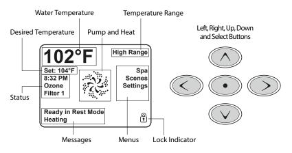
Set Temperature can then be adjusted with the up and down buttons. Pressing the Select button or the Right Arrow button will save the new set temperature.
