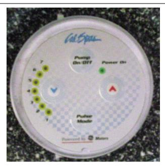
Figure 15. Adjustable Therapy System<sup>TM</sup> seatside control
