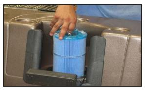
Unscrew the cartridge and remove it.
