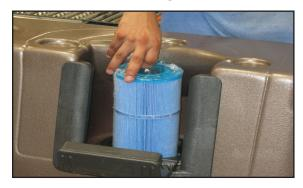
Unscrew the cartridge and remove it.
