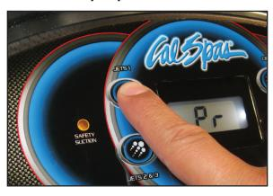
Your spa will perform a self-diagnostic check and go into priming mode. When the control panel displays **PR**, do the following:
