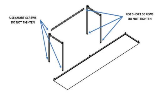
E. Place other side leg into top then place cross bar between side leg and center leg (11-foot model)
