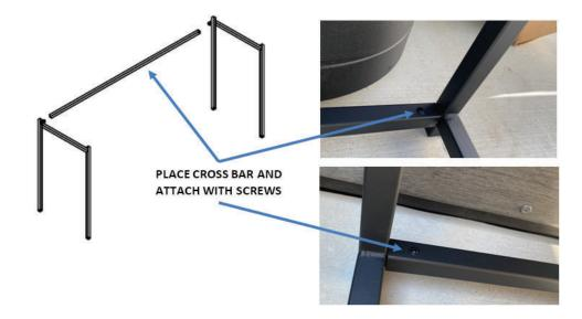
E. Use short screws to attach legs to bar top
