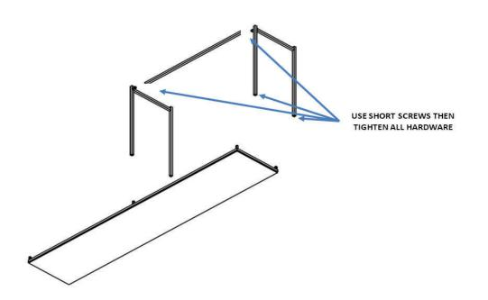
F. Use short screws to attach side leg and cross bar together and tighten all other hardware
