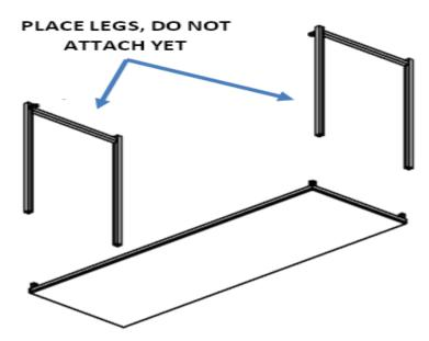
D. Place cross bar in place between legs and use short screws to attach all pieces together.
