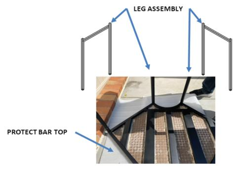
Use short screws to attach leg assemblies to corner bar D.
