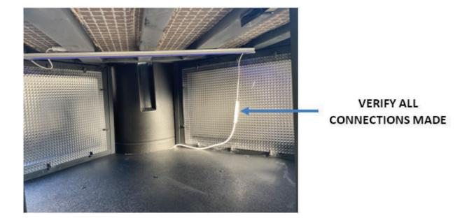
B. Route and dress cables using cable ties as required.
