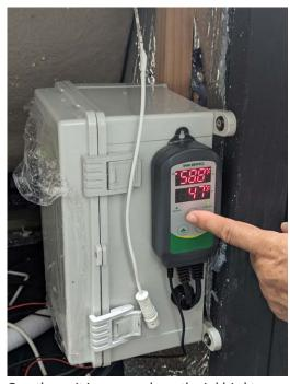
One the unit is removed use the inkbird temperature control unit and press and hold the set button
