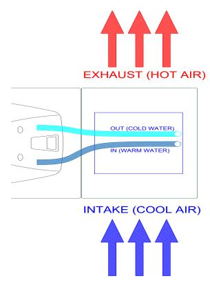
With any chiller or refrigeration system, when the ambient temperature is above a certain threshold, the heat generated by the refrigeration system has no where to go. This causes a problem where hot air is being used to cool down the unit when it is operating. When this occurs the water within the chill spa will still cool, but the rate of cooling is less than when the chill spa is operating in its ideal conditions below 90°F.
