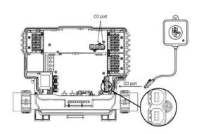
Simply connect the spa transmitter into an available CO port of the spa control system (or any other accessory with a free CO port, such as the in.stream 2 audio amplifier, or the in.clear water sanitization system).
