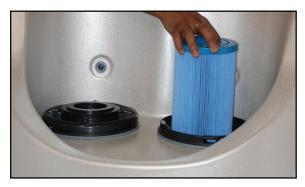
NOTE: After you remove the filter, remove the plastic wrapper and soak it in water for 30 minutes before you replace it. A dry filter can allow air into the filtration system which can cause the pump to fail to prime. Never try to pull the filter cartridge while the spa is running in low or high speed (i.e., any speed).
