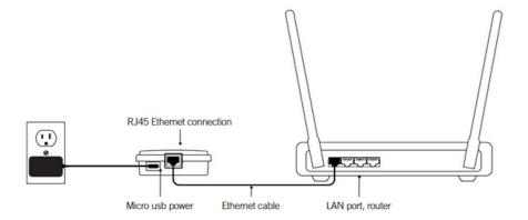
Simply connect the ethernet cable into the RJ45 port of the in.touch 2 home transmitter and in one of the available LAN ports on your router. To power up the home transmitter, plug the provided wall outlet charger to a 120V (North American model) or 220V (European model) household supply and connect the USB cable to the wall outlet and the home transmitter.
