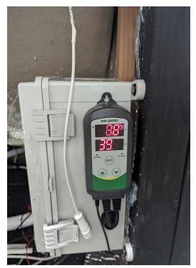
Select your lowest temperature, use the up or down arrows to adjust set point, the lowest the unit can support is 39F°. Once set press "set" to save the adjustment a HD will appear after a successful temperature adjustment.
