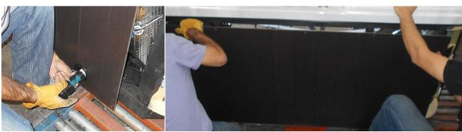
Reach in and pull the drain assembly through by a few inches. Carefully unscrew the black outer drain knob and then unscrew and remove the front door panel.
