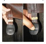
**Step 3** - With the straps pulled taut (but not overly tight), lightly drill the location for screw placement. Gently drill 3 holes - one for each screw slot in the lock. (If you do not have a low torque drill, use the lowest torque setting on the drill you have.) DO NOT drill all the way in but instead just make a guide for starters.
