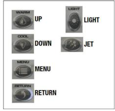
Default Timeout setting: Spa LIGHT is 60 minutes; BLOWER is 15 minutes, JET at low speed is 60 minutes; and JET at high speed is 15 minutes. User can change these default times in DEVICE TIMEOUT setting menu.
