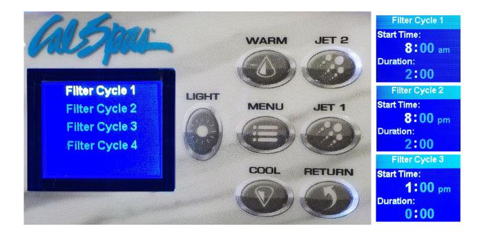
Filter Cycles 1, 2, 3 and 4 can all be adjusted in 15 minute increments. Use the MENU button to move from field to field, use the UP and DOWN arrows to make adjustments and then press RETURN once you're satisfied with your selections for all Cycles. Please note that the system will not allow you to set overlapping or contradictory Cycles.
